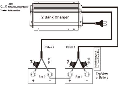
Two 12 VDC Batteries connected with a series jumper for a 24 VDC Trolling Motor
