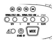
The state-of-charge (SOC) LED display has four (4) SOC indicators.
